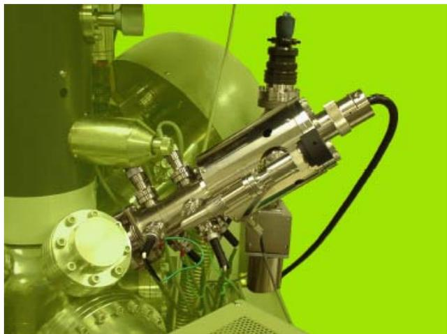
Figure: Floating micro ion etching device
