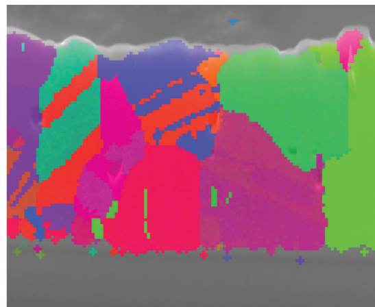
6. (a) Back-scattered image of a thin metal coating on glass; (b) EBSD map of the sample.
