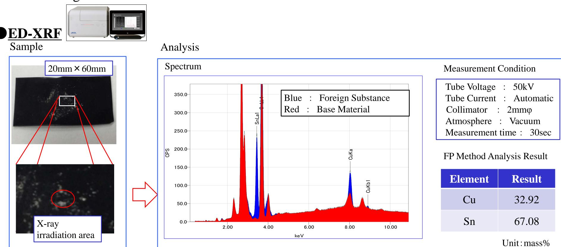
From the elemental analysis result, the existence of Sn and Cu can be confirmed. However, there is no steel grade which corresponds to the results obtained by easy quantitative analysis with the FP method. To make a detailed analysis of this steel grade, we conducted EDS elemental mapping by SEM-EDS.
