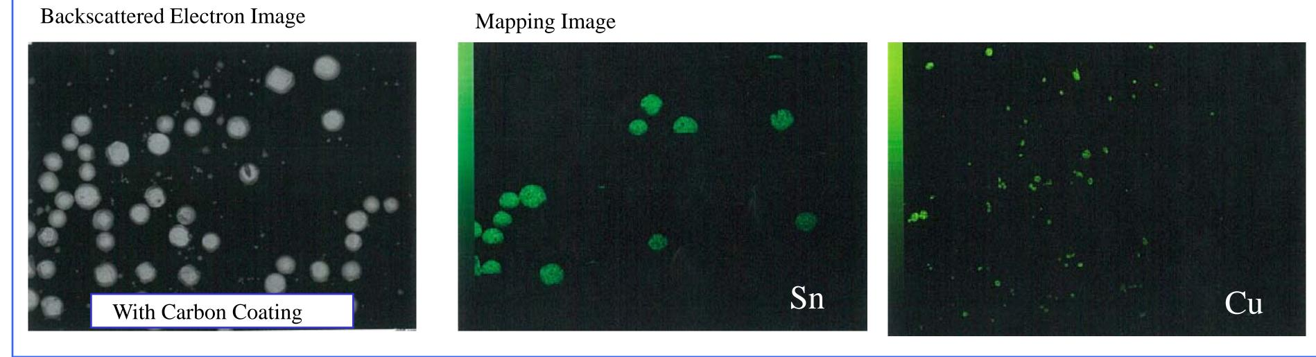
The existence of two different particles can be confirmed from backscattered electron image of **SEM-EDS.** Using EDS mapping image of each particle it was found out that smaller particles were Cu, and the larger particles were Sn.
