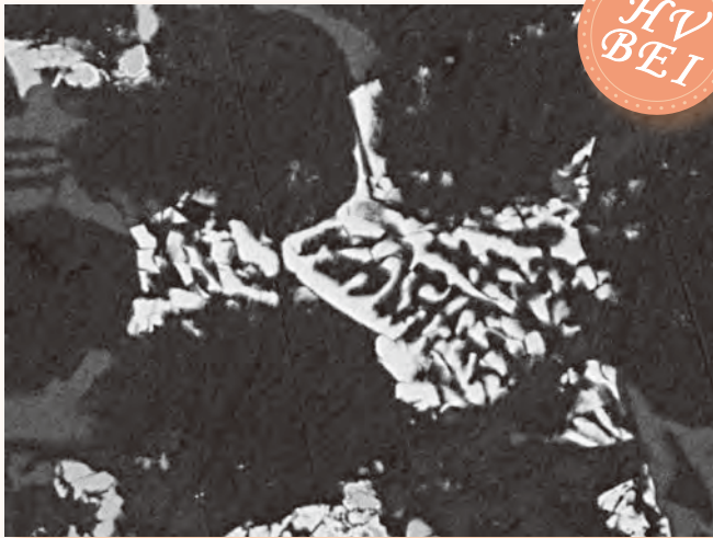
Sample: Aluminum alloy 10 \mu\text{m} Backscattered electron image Accelerating voltage 10 kV, magnification 3,000 \times
