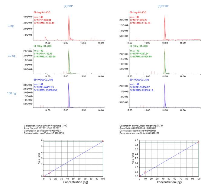
Figure 5 EICs chromatograms and calibration curves (Left : DBP, Right : DEHP)
