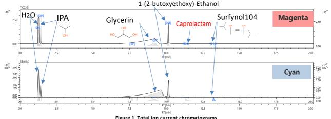
Figure 1 Total ion current chromatograms
